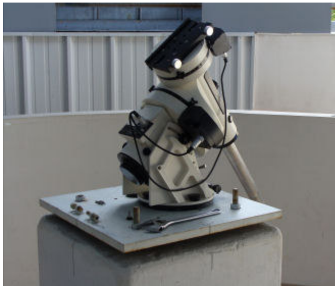
Equatorial mount of HCAS 14" Celestron, just before removal from pedestal, to prepare for observatory upgrades.
