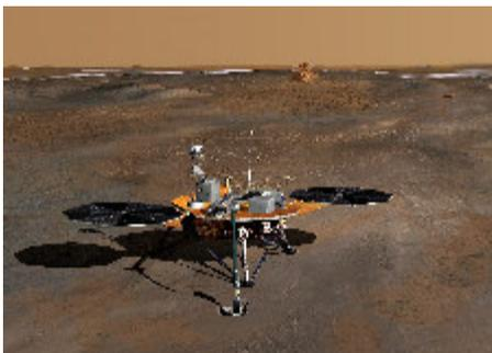
Phoenix will fly to a site farther north than any previous Mars landing. The solar-powered lander will robotically dig to underground ice and will run laboratory tests assessing whether the site could have ever been hospitable to microbial life. The instruments will also look for clues about the history of the water in the ice. They will monitor arctic weather as northern Mars' summer
