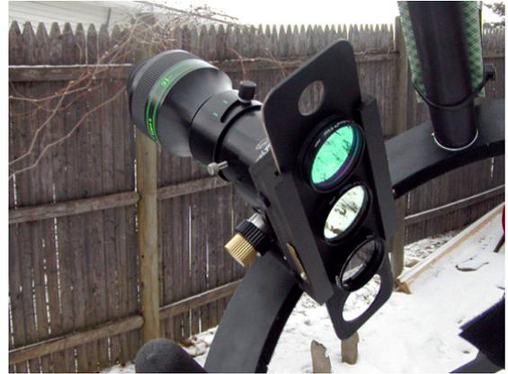
*A filter slide provides safe and easy access to your filters. Photo used with permission. [www.Astrocrumb.com](http://www.Astrocrumb.com)*
